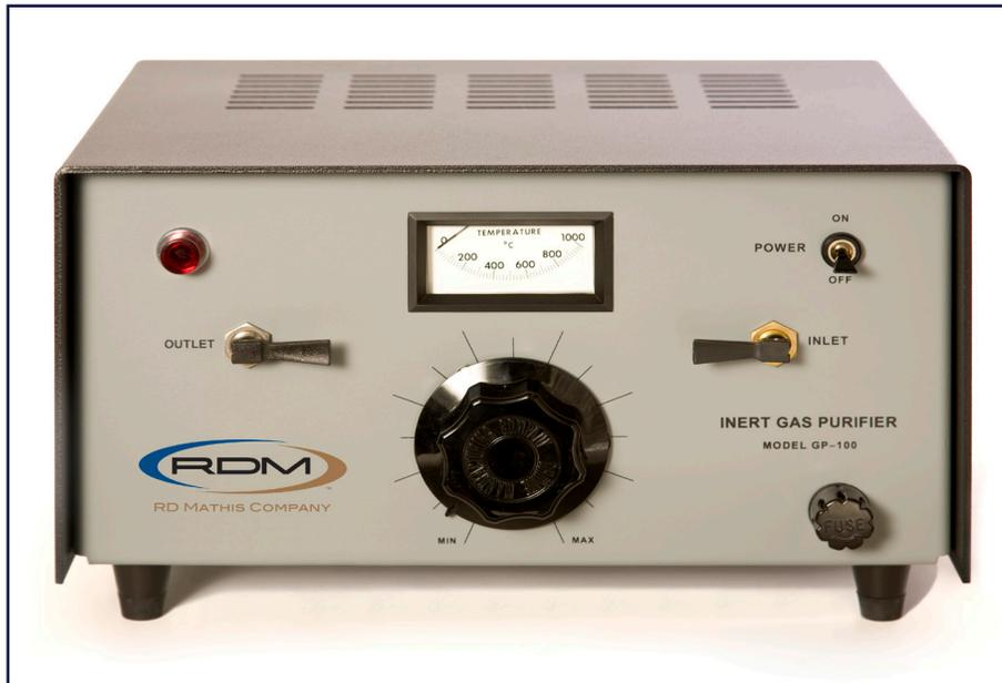
The GP-100 has been shown to purify 99.8% argon gas to 99.9991% purity as part of a worst case test. The principle impurity levels at flow rates of 1/4 liter/min. (0.53 cu. ft./hr.) were measured to be H<sub>2</sub> 0-2 p.p.m., N<sub>2</sub> /CO-3 p.p.m., O<sub>2</sub> -2 p.p.m., Ethane-1 p.p.m., other Hydrocarbons - no detection, and CO<sub>2</sub>-1 p.p.m., with the limits of detectability set at 1p.p.m.\*
